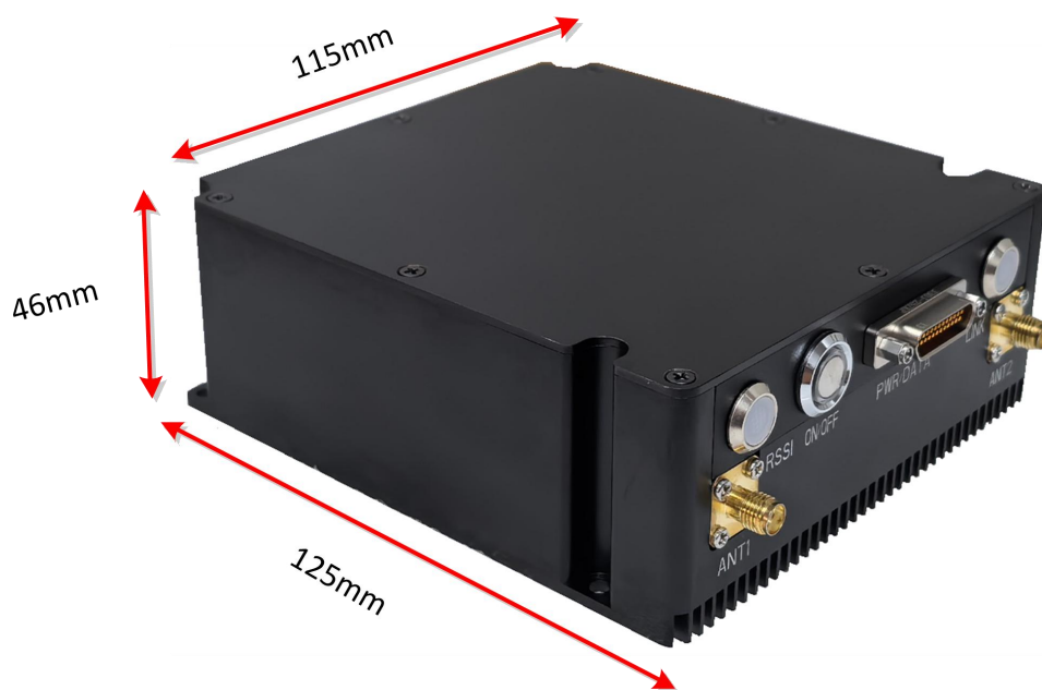
Fig. 4.1 Physical picture and dimension of XK-M505E
